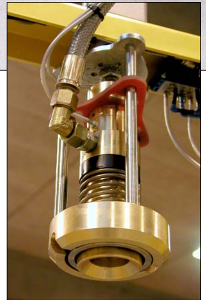
Fully automatic AFH filling head for centre valves
