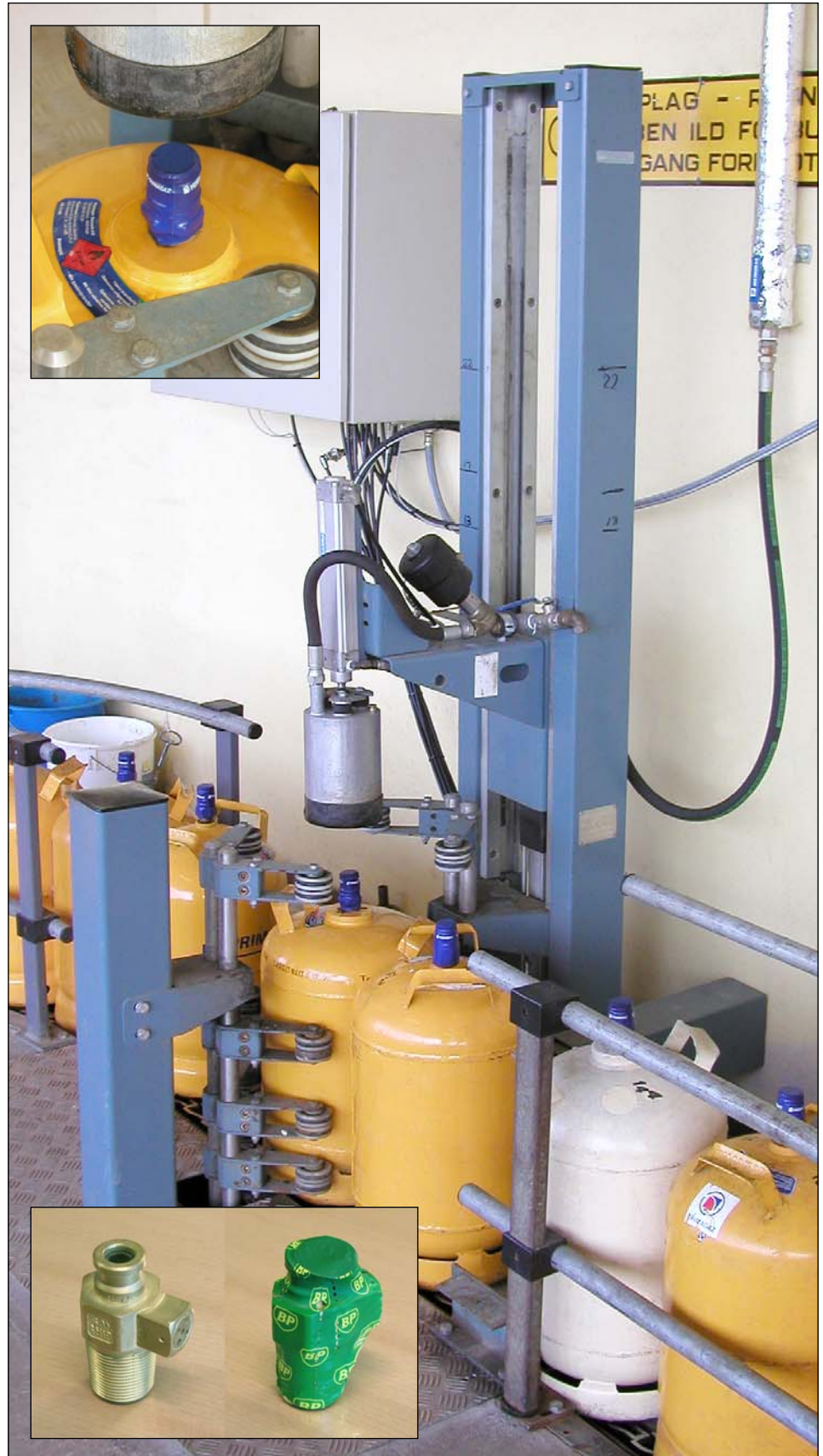
The fully automatic SMS thermosealing machine, which shrinks seals by means of water steam, is designed for installation in a chain conveyor
