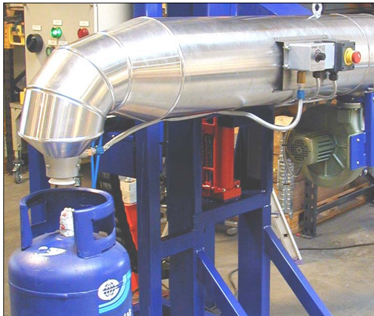
The fully automatic SMA thermosealing machine, which shrinks seals by means of hot air, is designed for installation in a chain conveyor
