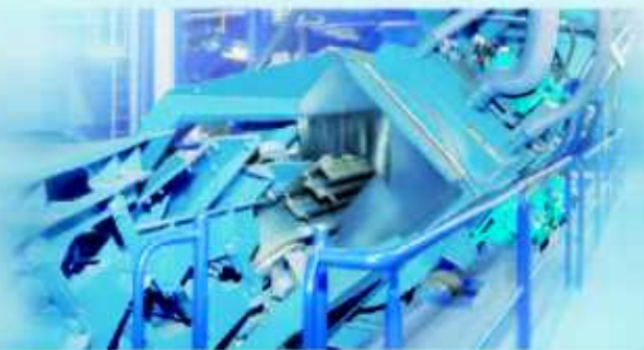
Loading zone of a CBC 10/30-450 shot blast machine
