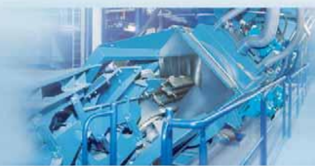
Loading zone of a CBC 10/30-450 shot blast machine
