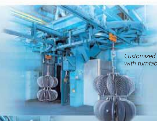
HT overhead monorail shot blast machine for descaling
